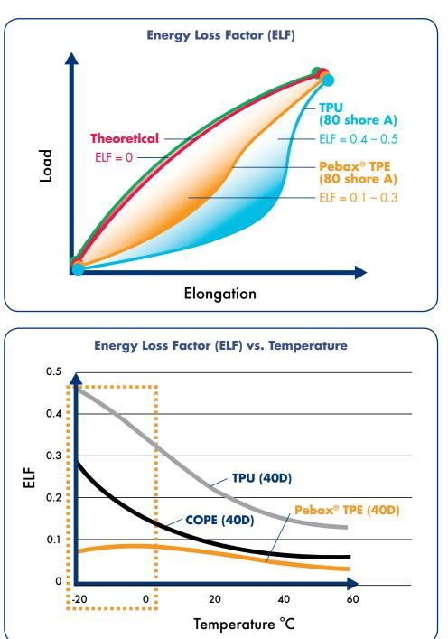
For industrial belts and silent gears the lower hysteresis (higher energy return) of Pebax<sup>®</sup> resins can translate into higher speed and frequencies of use and even subsequent energy savings through better power transmission and low heat buildup.
